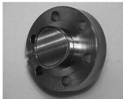
Figure 1: Cross-section and photo of an LHC button.
