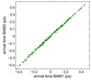
Figure 16: EO Arrival time monitor 9.5fs RMS difference over 1 minute measurement at DESY / FLASH.
