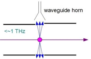
Figure 4: Waveguide based pickoff.
