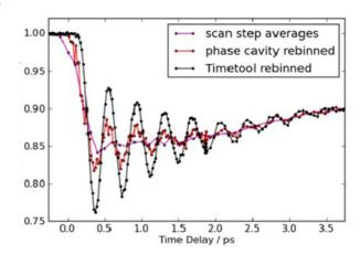
Figure 10: X-ray / Optical correlator (Time tool) improves resolution for non-thermal melting of Bi.[11]
