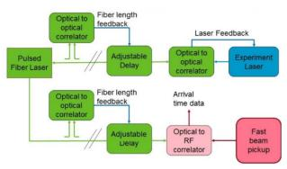
Figure 14: Fiber timing backbone.
