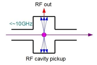
Figure 3: Cavity pickup.
