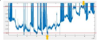
Figure 13: Drift over 2 week measurement ~340fs pk-pk.
