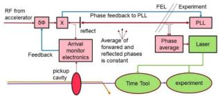
Figure 11: LCLS timing system overview.
