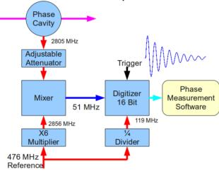
Figure 12: Arrival time processing electronics.
