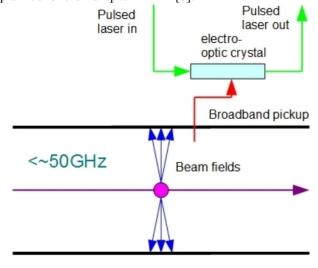
Figure 6: Indirect EO sampling.
