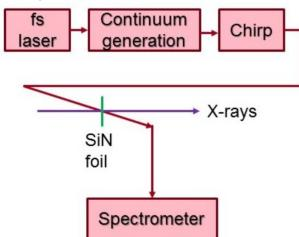
Figure 9: X-ray/optical cross correlator at SLAC/LCLS.
