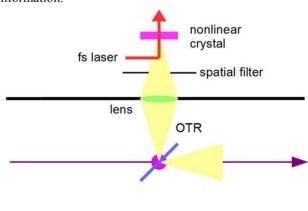
Figure 8: OTR signal generation.
