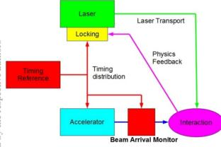
Figure 1: Typical timing system
