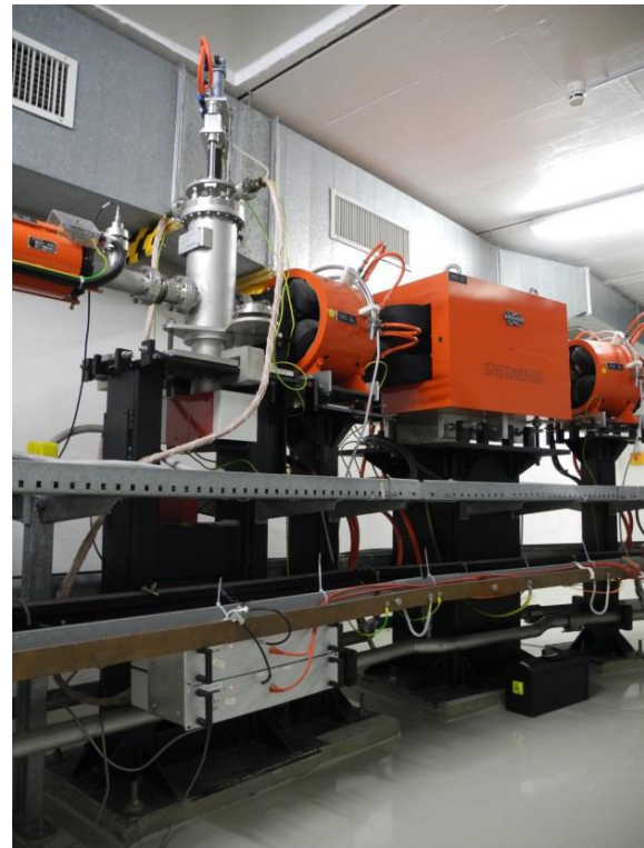
Figure 4: Harp station 4 in the IBL contains a vertical and a horizontal harp moved by one pneumatic drive. Two multichannel pico-amperemeters are mounted below the cable tray.
