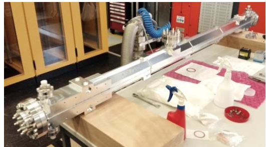
Figure 8: IBFB kicker magnet during vacuum acceptance test at PSI.
