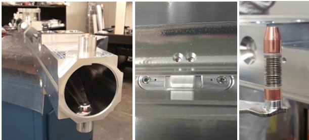
Figure 5: IBFB kicker magnet during assembly. Left: Kicker magnet without end flanges. Middle: Sliding ceramic spacer (white) allows relative movement of strip and outer vessel. Right: Flexible RF feed-through at end of strip.
