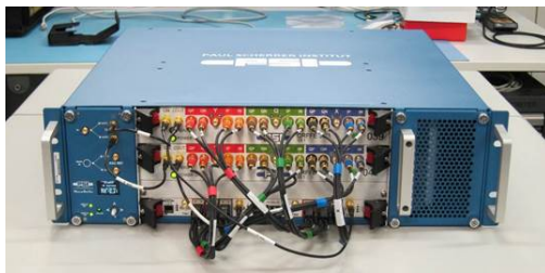
Figure 2: E-XFEL cavity BPM electronics (MBU = Modular BPM electronics), with two cavity BPM RF front-ends (RFFEs, top) and FPGA carrier board with two ADC mezzanines (bottom) [2].
