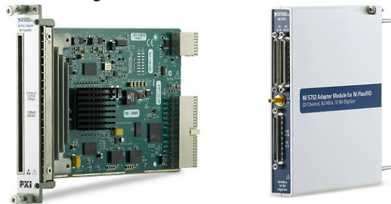
Figure 4: PXI-7954R FPGA card and NI-5752 Digitizer Adaptor Module.
