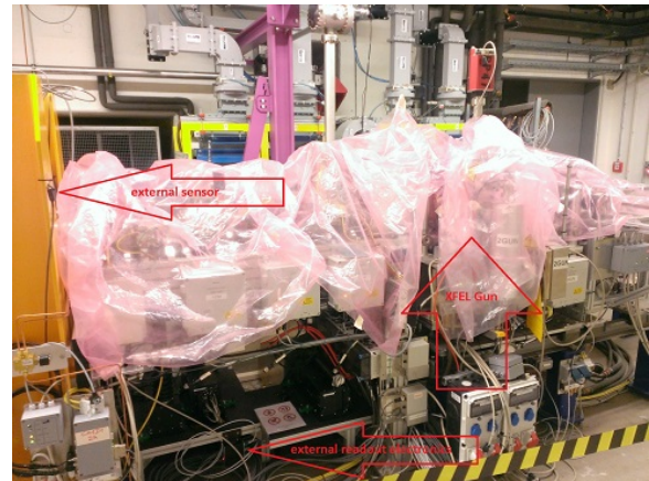
Figure 3: external readout module and sensor at the XFEL Injector.
