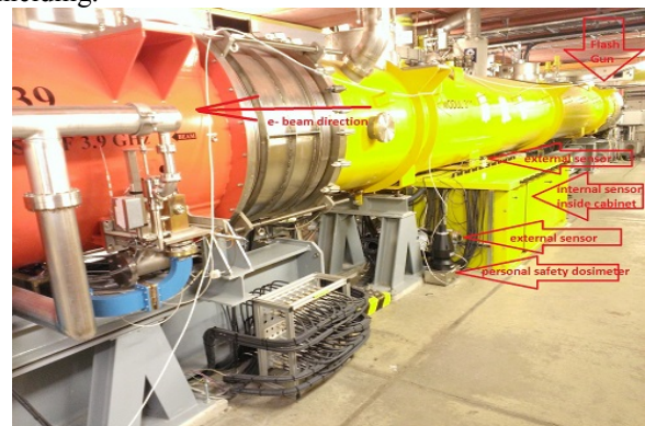
Figure 4: full system setup at Flash RF-gun rack.
