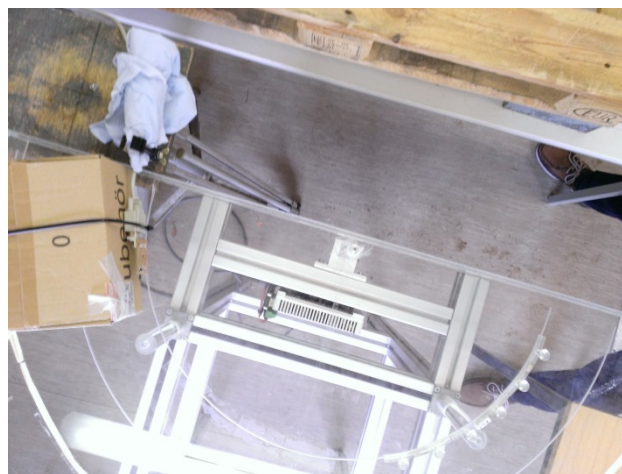
Figure 7: Cs-137 calibration setup (top view).
