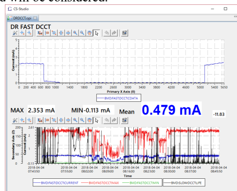
Figure 2: Example of DCCT data of DR with accumulation time of around 1 ms.
