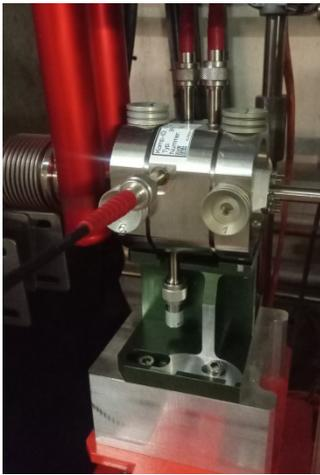
Figure 5: Cavity BPM in the FLASHForward beamline.
