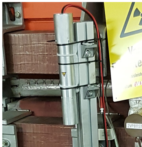
Figure 3: BLM prototype based on a scintillator and PMT setup during tests in the COSY synchrotron.
