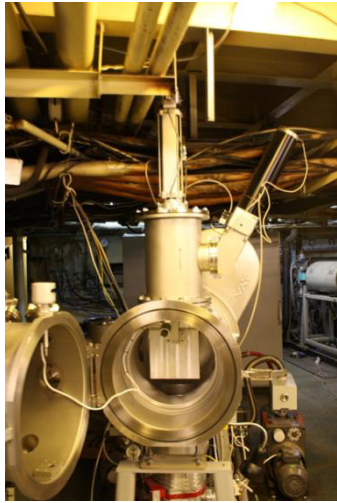
Figure 2: Wide-angle complete-overlap ion beam profile monitoring system (installed in the beam channel).
