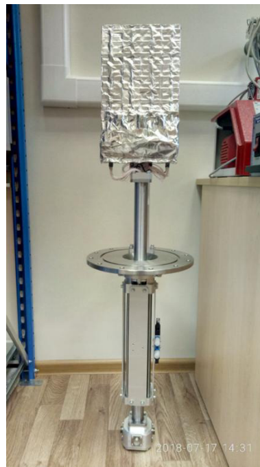
Figure 1: Wide-angle complete-overlap ion beam profile monitoring system (ready-assembled, before installation).
