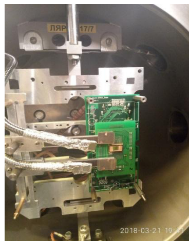
Figure 7: Positioning of scintillation online detectors system for test support on the DUT.
