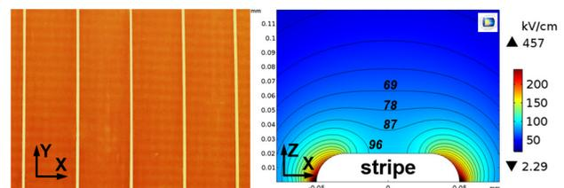
Figure 3: Photo of 100  $\mu\text{m}$  stripes at the FR4 plate and distribution of electric field near a stripe at -4 kV potential.
