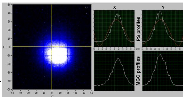
Figure 9: Beam cross-section at the PS and postprocessing profiles from the PS image and from MGC data.
