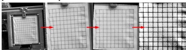
Figure 5: Image correction procedure in NI Vision.
