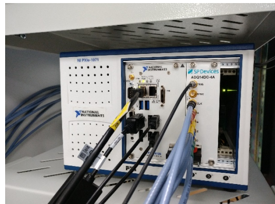
Figure 1: Data acquisition board and PXIe chassis for BTB position on-line measurement.
