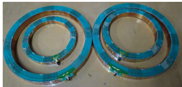
Figure 5: FCTs and ICT tied up to a 16-turn 8-direction coil with a 50 \Omega PCB board.
