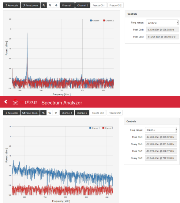
Figure 2: Tests for spectrum API: The upper one is tests in Laboratory with signal at 667kHz & 220mV; The bottom one is tests in the BEPCII IP Station, in which the peak frequency 624 & 638kHz both correspond to the X tune in BEPCII.
