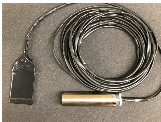
Figure 2: BC408 scintillating detector and optical fibres with light proof covering, connected to a Photo Multiplier Tube (PMT).
