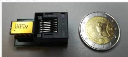
Figure 6: RadFET chip mounted on its PCB with RJ45 connector.
