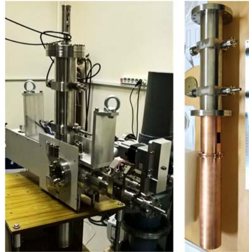
Figure 8: Photo of assembled BSM with the magnetic shield and symmetric RF-deflector.
