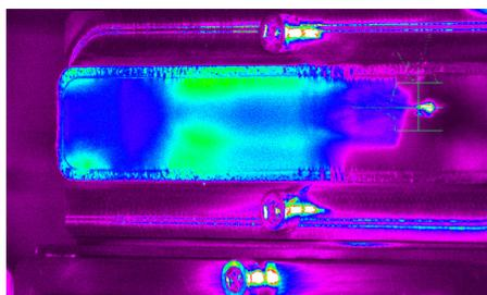
Figure 6: Electron beam imaging on OTR screen.
