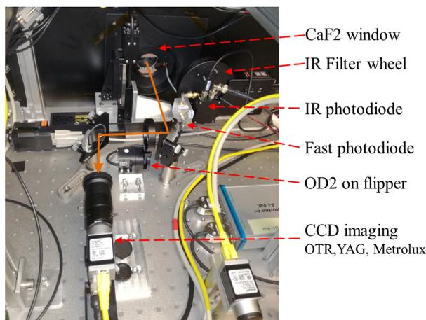
Figure 5: Layout of optical components and detectors.
