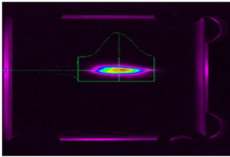
Figure 7: Seed2 laser spot imaging on Metrolux scintillator.
