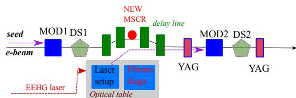
Figure 1: Layout of EEHG experiment at FERMI.
