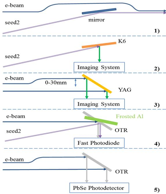
Figure 2: Diagnostics configurations.
