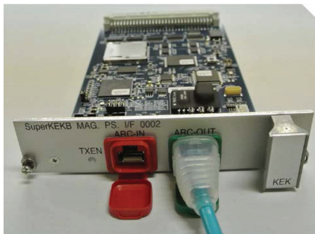
Figure 5: Prototype of the PSICM (Power Supply Interface Controller Module), used for the magnet power supply control for SuperKEKB.
