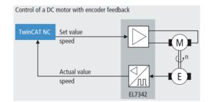
Figure 2: Beckhoff TwinCAT NC axis velocity control loop.
