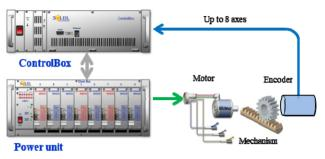
Figure 1: Standardized hardware architecture.
