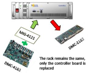
Figure 4: Replacement controller of into CONTROLBOX.
