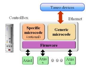
Figure 2: Microcode and Tango devices.
