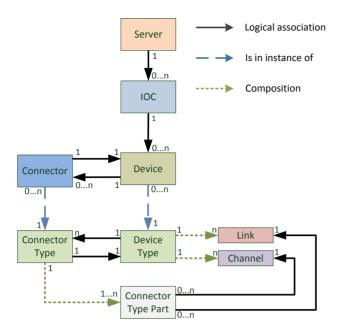
Figure 1: Data model of NSLS-II Booster magnetic subsystem.
