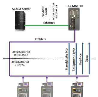
Figure 5: Mobile Controllers Fieldbus.
