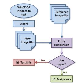
Figure 2: The procedure for validating a test instance of an ECAL DCS application against a valid reference.
