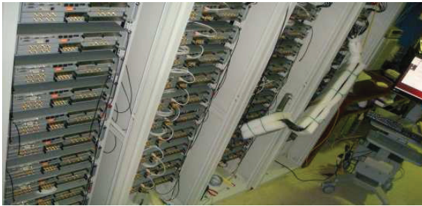
Figure 3: All TPS BPM testing in the TLS booster area.
