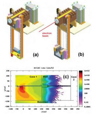
Figure 2: beam deflector for straight forward beam lines: (a) IN position (b) OUT position (c) radiation distribution from maximum beam power to be dumped.
