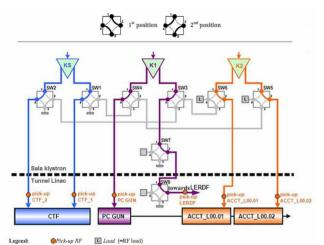
Figure 2: Layout of the waveguide switch system of the first part of the linac.
