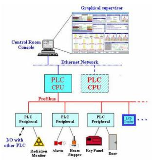
Figure 4: Block diagram of the safety systems architecture.
