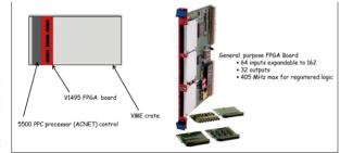
Figure 6: V1495 FPGA board.
