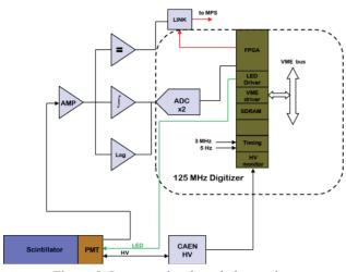
Figure 5: Loss monitor board electronics.
