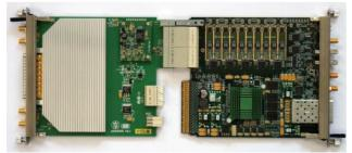
Figure 1: Pair of MTCA boards connected via Zone 3.
