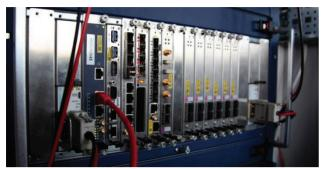
Figure 2: MTCA.4 crate in operation at DESY.
