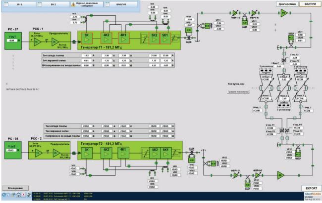
Figure 3: The video frame of functional diagram of RF-system of the main ring KSRS.
