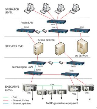
Figure 1: Structure of RF-generators CS.
