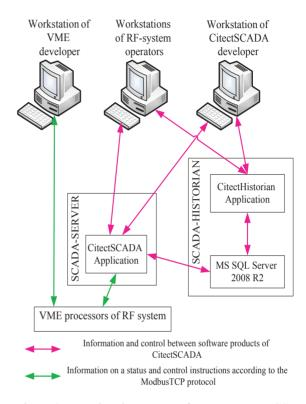
Figure 2: Functional structure of RF-generators CS.
