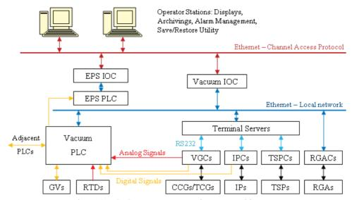
Figure 1: NSLS-II vacuum control system architecture.
