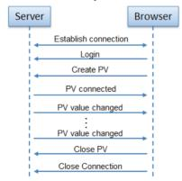
Figure 3: Typical communication sequence of WebPDA.
