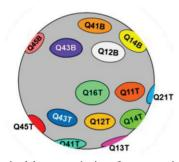
Figure 3: Typical beam pointing for cross-timing shot as viewed from the equator of the target chamber at  $78^{\circ}$  azimuth. All 4 beams in each quad are pointed to the same spot.
