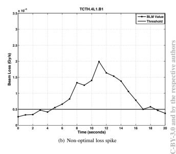
Figure 2: Optimal beam loss spike generated by the TCSG.B5L3.B2 collimator (left) and non-optimal beam loss spike generated by the TCTH.4L1.B1 collimator (right). A BLM threshold of  $5 \times 10^{-6}$  Gy/s was set in each case.
