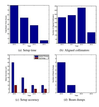
Figure 5: Summary of the performance gains with automatic alignment.
