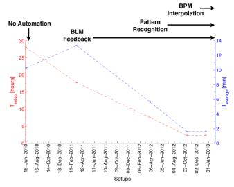
Figure 3: Evolution of  $T_{\rm setup}$  and  $T_{\rm average}$  for full alignments at flat top over the 2010-2013 LHC run.
