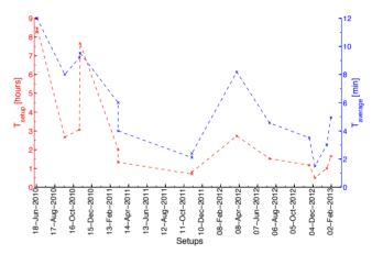
Figure 4: Evolution of  $T_{\rm setup}$  and  $T_{\rm average}$  for TCT alignments with squeezed separated and colliding beams over the 2010-2013 LHC run.
