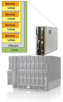
Figure 2: VMware still required a hosting OS (eg.Linux) on each HP Each Blade Server.
