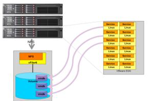
Figure 5: Using a virtual NFS server to store virtual disk images for virtual machines.
