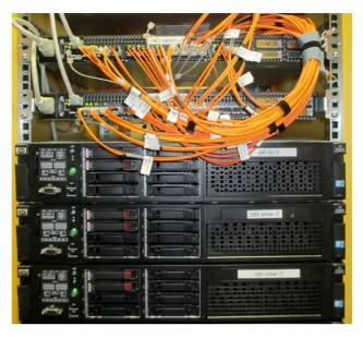
Figure 3: Cluster with 3 HP Intel servers and full redundant FC connectivity across two Qlogic switches.
