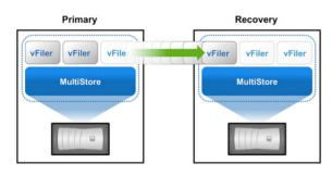
Figure 4: MultiStore enables you to migrate or back up data from one storage system to another without extensive reconfiguration on the destination storage system.
