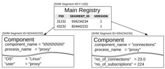
Figure 1: CMX's data structures in System V Shared Memory.
