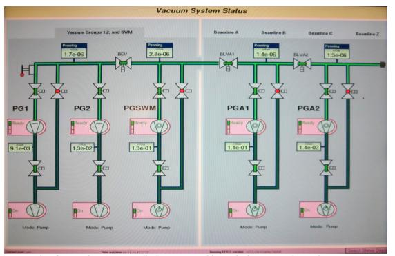
Figure 1: Example of an engineer's status display screen. This particular screen shows the vacuum system status, pressures, meters, valves. Other screens are available via a popup menu indicated at lower right.
