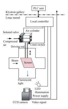
Figure 2: Block diagram of the screen monitor system in the KEK injector linac.
