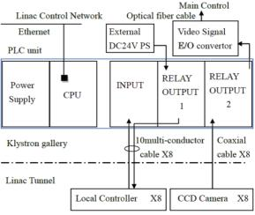
Figure 5: Block diagram of the PLC-based screenmonitor control system.
