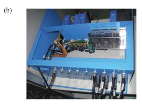
Figure 4: Photograph of the PLC-based screen monitor control system, (a) front view and (b) rear view.
