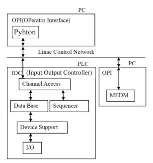
Figure 6: Flow chart of the control software in the PLC.
