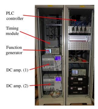
Figure 3: Control rack of skew quadrupole magnets.
