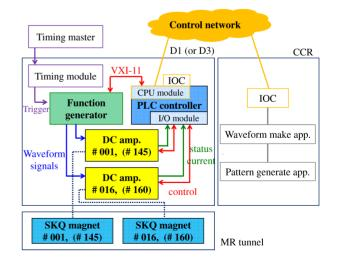
Figure 2: Devices of the SKQ control system.
