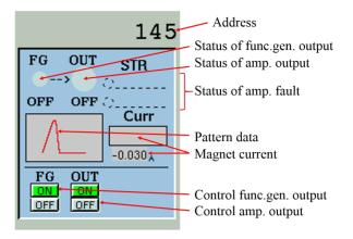
Figure 4: Control screen for SKQ magnet setup.
