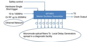
Figure 3: Central Master Transmitter interface.
