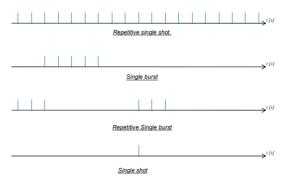
Figure 4: User-programmable laser shot sequences.
