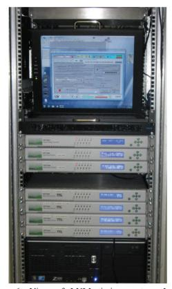
Figure 6: View of LULI timing system. In this installation the users have measured the long-term jitter in a temperature stabilized environment. The results are shown in Figure 7.
