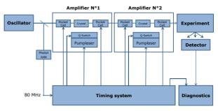
Figure 1: Typical picoseconds laser system.
