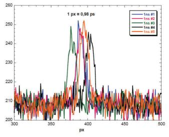
Figure 7: Result of timing system jitter.
