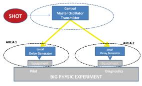
Figure 2: Timing system architecture.
