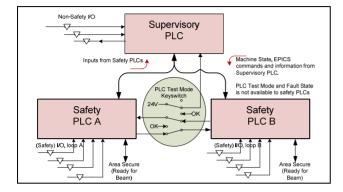
Figure 1: The typical architecture of SLAC safety systems.
