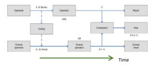
Figure 3: Time redundancy and diversity achieved in a single failsafe CPU.
