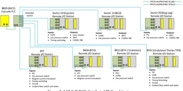
Figure 2: LCLS-II BCS distributed PLC architecture.
