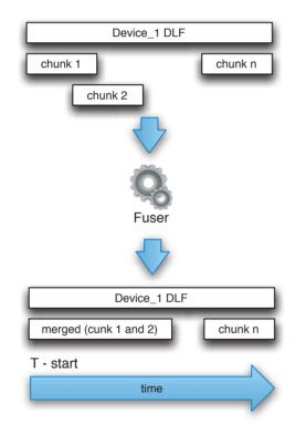
Figure 3: The "Chunk Fusion" logic.
