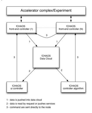
Figure 1: Data exchange between components by means of !CHAOS Data Cloud.
