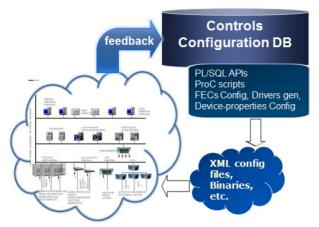
Figure 1: Overview of the configuration data flow.
