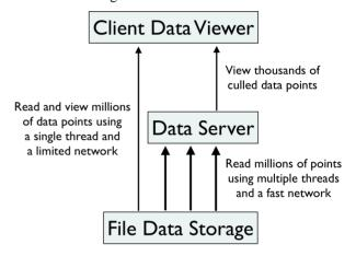
Figure 1: Benefits of using an intermediate Data Server vs. reading and displaying data directly from disk.
