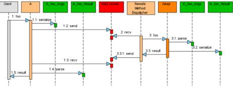
Figure 2: Sequence diagram of a synchronous client call.
