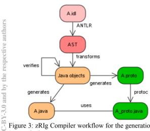
Figure 3: zRIg Compiler workflow for the generation of a Java stub class.
