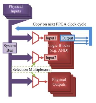
Figure 4: FPGA System Bus.
