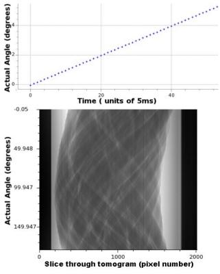
Figure 7: Example of tomography pulses and sinogram.
