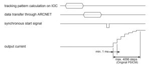
Figure 4: Schematic diagram of synchronous operation.
