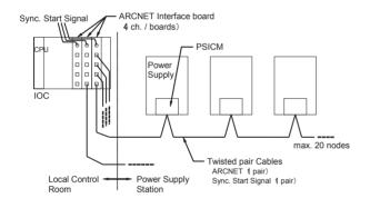
Figure 3: Typical configuration of ARCNET in KEKB.
