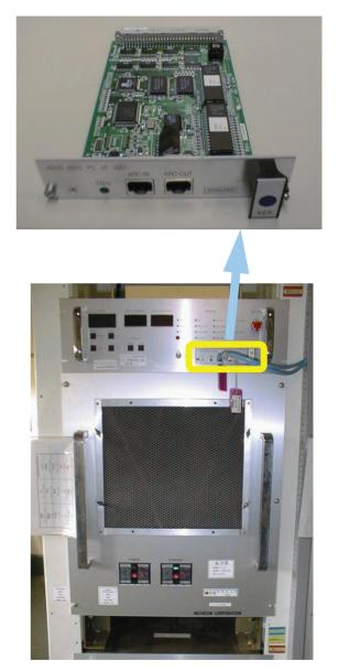
Figure 1: whole shape of the PSICM (above) and the PSICM plugged in a magnet power supply (below).
