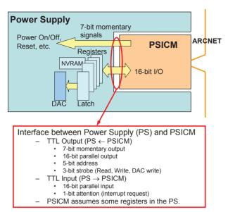
Figure 2: The interface to the magnet power supply.
