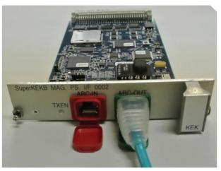
Figure 5: Prototype of the new PSICM.
