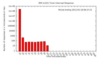
Figure 2: Timer interrupt latency for LX25 hardware.
