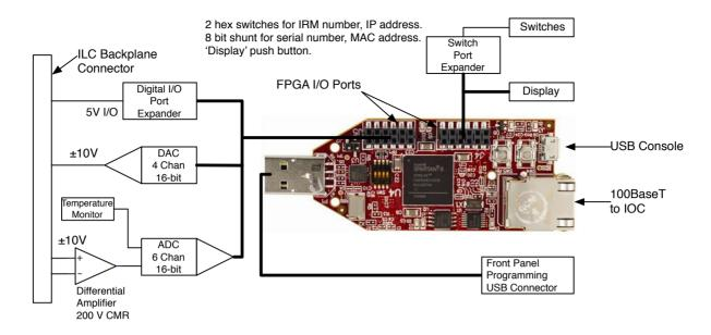
Figure 1: IRM hardware showing commercial FPGA board and added components.
