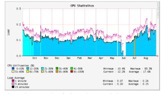
Figure 3: Example of Linux CPU statistics (gaps due to reboots or OpenNMS monitoring restarts).
