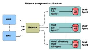
Figure 1: Example of a SNMP architecture [4].
