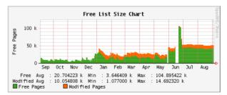
Figure 2: OpenNMS memory chart showing very low free memory (green), and the installation of a secondary page file (orange). Gaps are due to system downtime.
