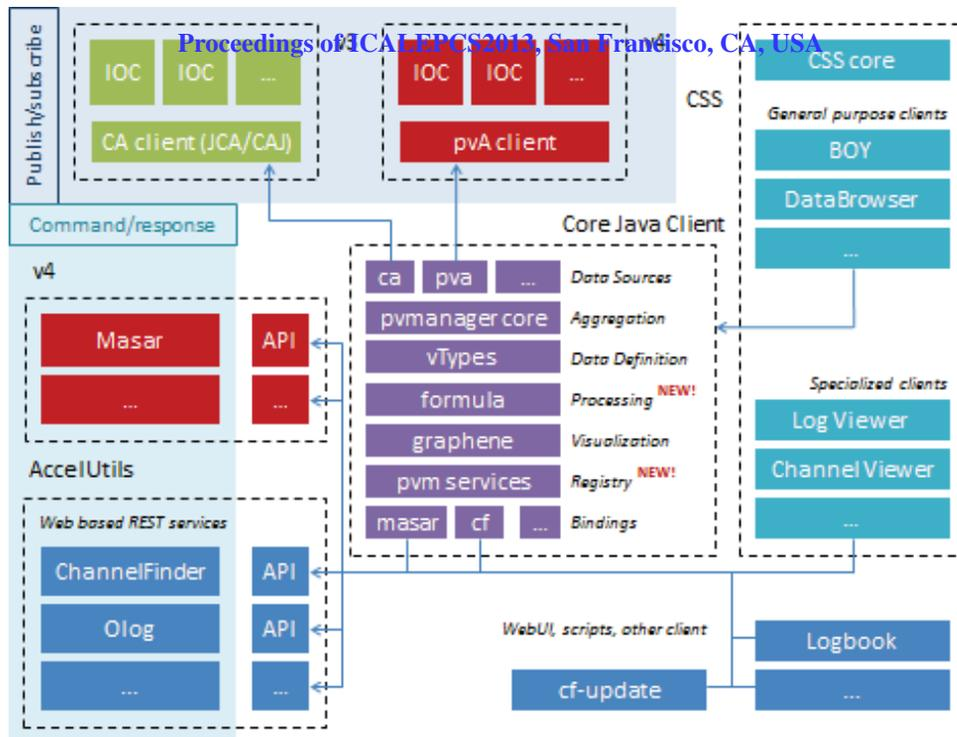
Figure 2: Overall Architecture of accelerator tools and services.
