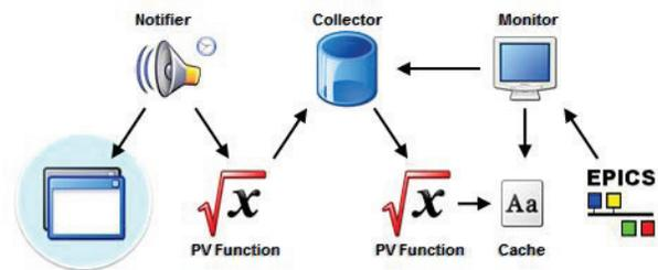
Figure 1: Architecture diagram. Shows the part of the client that runs at the rate dictated by the source of the data on the right and the part of the client that runs at the rate at a client dependent rate.
